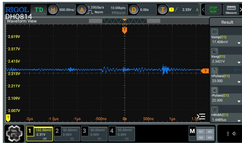
Figure 4: Sub-1 \mu s noise window. Baseline 2.3421 V; Vamp 17.408 mVpp; width 1.4485 \mu s.
