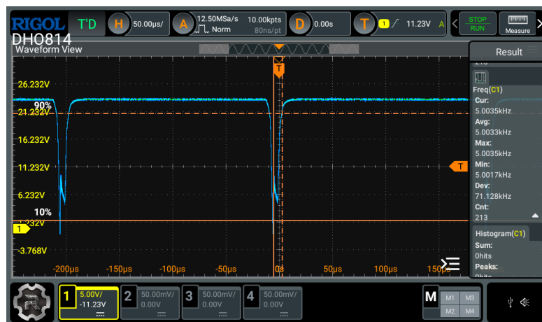
Figure 3: Full-scale waveform. Freq 5.0035 kHz (avg 5.0033 kHz, dev 71.128 Hz); amplitude +26.232 V to – 3.768 V.
