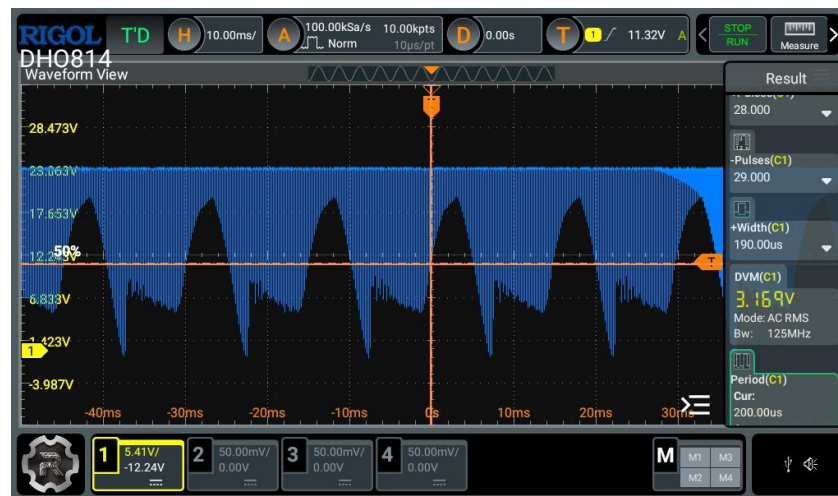
Figure 2: 10 Hz burst envelope of the 5 kHz carrier. Pulse width 190 \mu s; 29 bursts captured; AC RMS 3.16 V.
