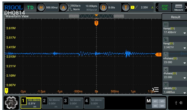
Figure 4: Sub-1 \mu s noise window. Baseline 2.3421 V; Vamp 17.408 mVpp; width 1.4485 \mu s.
