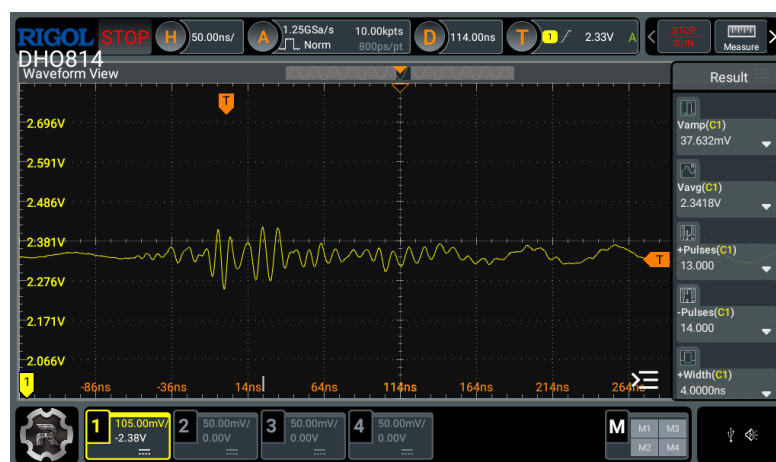
Figure 5: Edge-transition ringing. Vamp 37.632 mV; Vavg 2.3418 V; decay < 150 ns.
